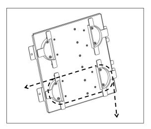
Figure 11. Cable take-up reel routing
