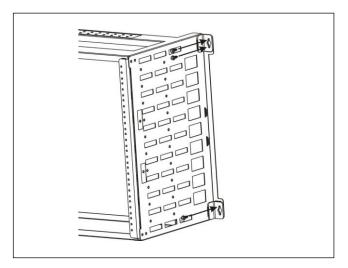
Figure 6. Mounting screw locations
