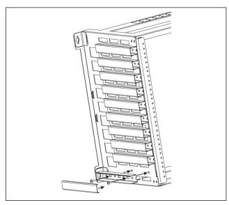
Figure 8. Cable guide installation
