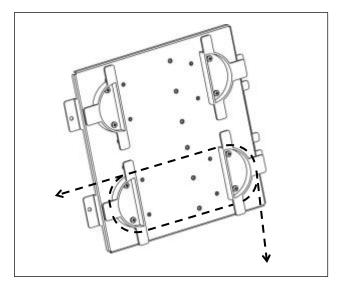
Figure 11. Cable take-up reel routing
