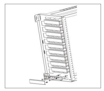
Figure 8. Cable guide installation
