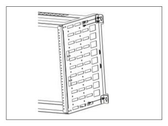
Figure 6. Mounting screw locations
