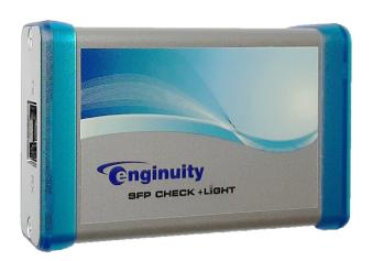
For dark fiber qualification, plug an SFP into the SFP CHECK+LIGHT to provide a light source. Use an optical test set to measure the optical power levels along a fiber optic path. Matching the wavelength of the SFP to any CWDM or DWDM splitters in the path enables a complete qualification at varying data rates.
