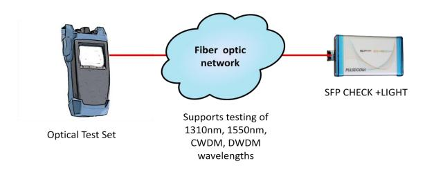
In addition, the SFP CHECK +LIGHT may be used to test SFPs. Connect the SFP CHECK +LIGHT to a laptop and display information such as Transmit Level, Receive Level, Temperature, Wavelength, and Data Rate.
